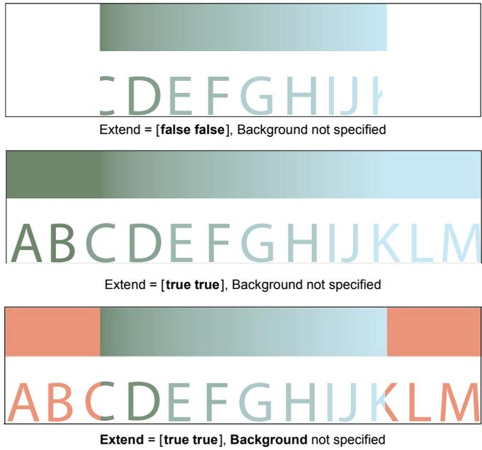
Figure L.10 – Axial shading (8.7.4.5.3, "Type 2 (Axial) Shadings")
